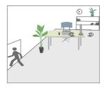
After the UVC lamp is powered on, when people leaves the scene, the lamp flashes 10s / 20s and then turn on the light.
