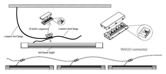
Step 3: Connect input cord to WAGO connector, then open the small plastic cover on both end caps of the batten light in order to connect each lamp together, finally fit the batten light to the clips on the ceiling.
