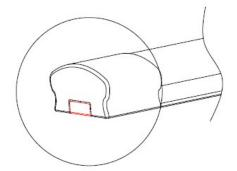
For Single unit installation, no need to open the end caps; For Linkable installation, need to open the end caps.
