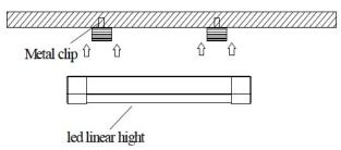
Step 4: Install batten light to the clip, fix the screw
